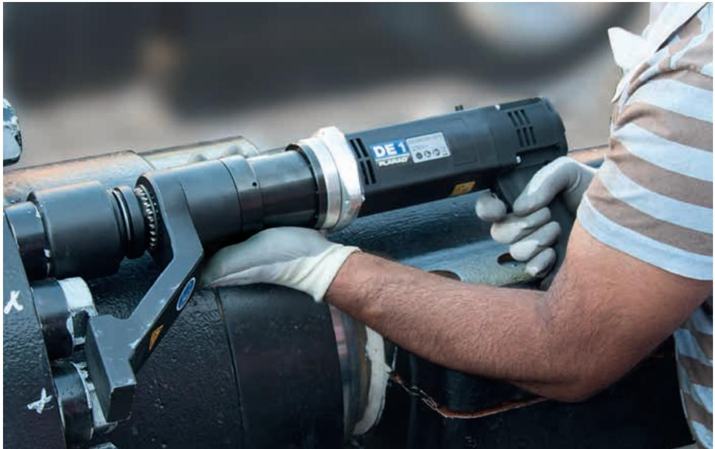
We have given the DE1 a new control system which includes voltage monitoring and speed sensing. This allows you to complete your bolting with even greater precision and reliability. As it reliably offsets any voltage fluctuations and changes in temperature, this new tool delivers superior torque accuracy. The DE1 switches automatically to the main available frequency (e.g. 50 Hz or 60Hz).
